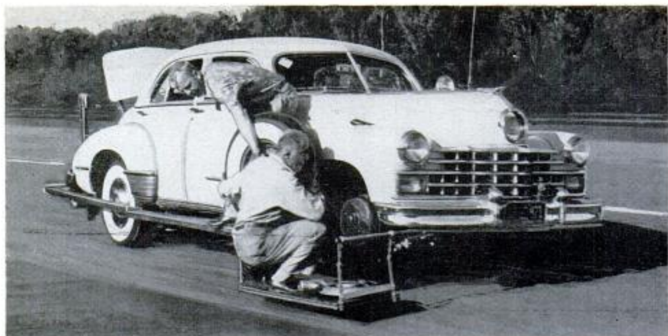
With the car going 20 m.p.h., Mattar removes the flat tire and puts on spare. Note running board to trunk
